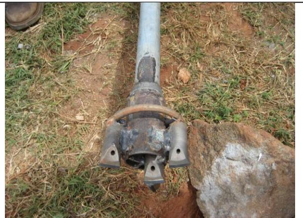
New drill bit using tungsten tips. These drill bits can drill hard layers like sand stone and laterite without getting blunt.
