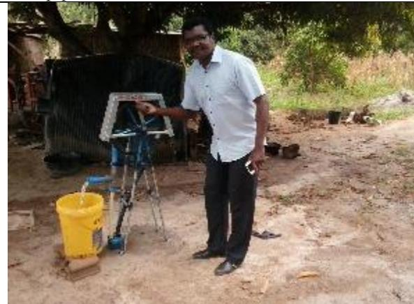
In this case in Maputo the 6 meters deep Tube was made in 1 day and a Rope pump is installed on a prefabricated slab
