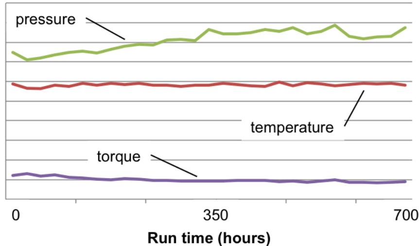
Figure 6. Laboratory test stand data for accelerated life testing of critical LifePump components. Results show the consistent water temperature, PCP element torque values, and flow rate. Testing conditions simulate 70 meters of depth. A comparison of results to field data validates the laboratory testing.
