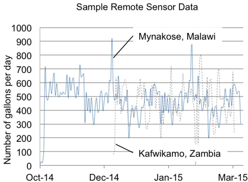
Figure 5. Satellite-based remote monitor data collected from two communities in Malawi and Zambia. The graph shows the number of gallons pumped per minute based on pumping efficiency and the number of handle rotations. This data is collected daily through satellite transmission and can be used by WASH organizations’ monitoring projects.
