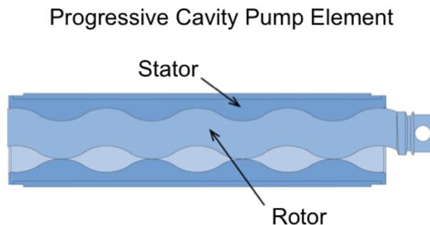
*Figure 2. The Progressive Cavity Pump (PCP) element consisting of the metal rotor and the elastomer stator. As the rotor turns inside the stator, pockets of water are pushed to the surface.*
