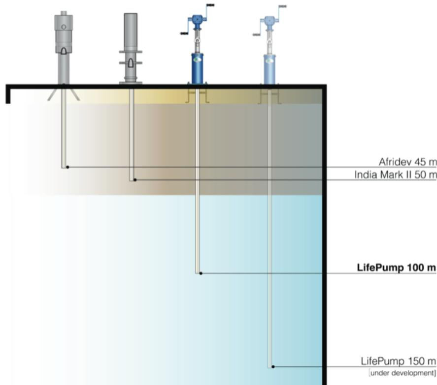
Figure 1. Depth comparison of the LifePump versus standard hand pumps Afridev and India Mark II. The LifePump currently reaches 100 meters, and a new model that will reach 150 meters is under development.
