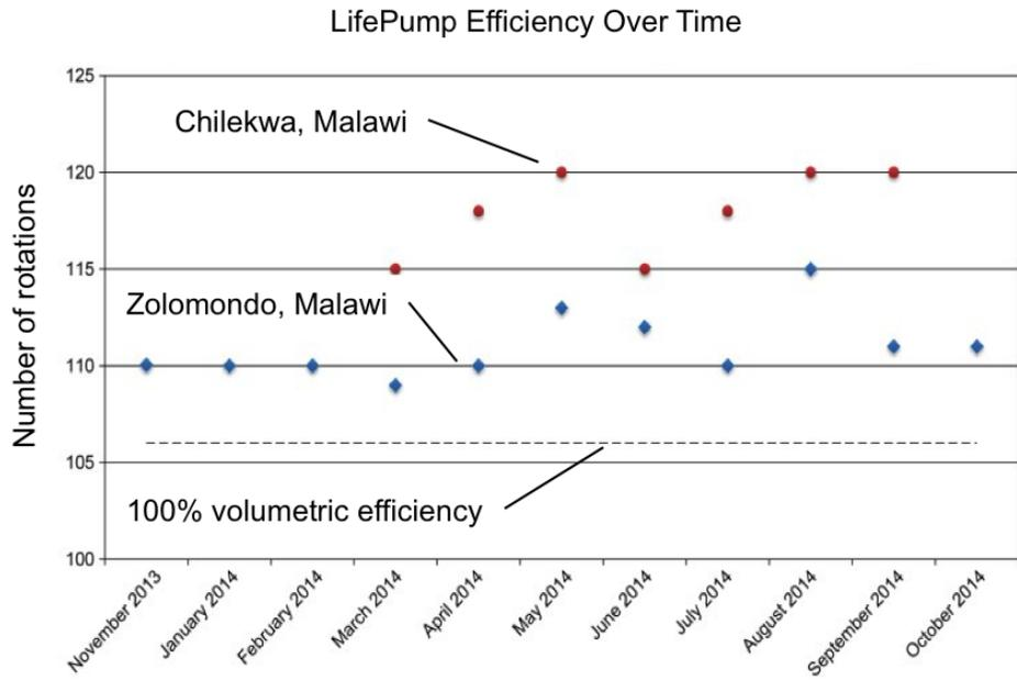
Figure 4. LifePump efficiency data collected from two communities in Malawi during the initial test phase of the LifePump pilot. The graph shows handle rotations required to pump 20 liters/~5 gallons. The 100% volumetric efficiency is shown, indicating a slight drop in efficiency as depth increases. The pump depths of Zolomondo and Chilekwa are 57 and 81 meters, respectively.
