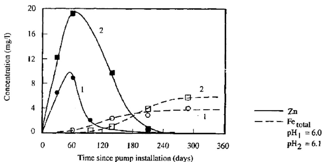
**Figure 1. Zinc (Zn) and total iron (Fe<sub>total</sub>) concentrations in groundwater versus time since installation of two non-corrosion-resistant handpumps (Moyno with galvanized rising mains and pump rods; Cote d’Ivoire). The iron concentration increases after the zinc peaks; that is, as soon as the protective coating (galvanization) is no longer intact.**
